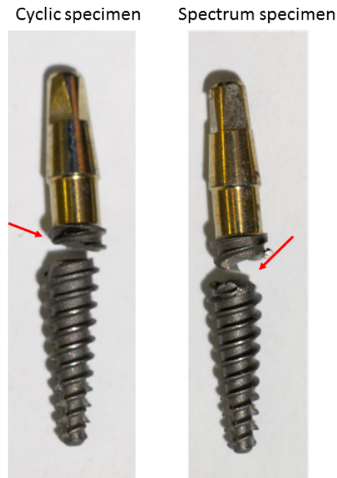
Figure 4: Fracture in the second thread of cyclic and spectrum loaded specimens.
