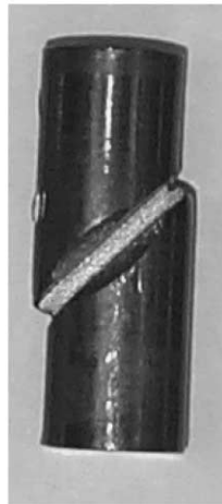
Fig. 1. Schematic representation of the SCS. All dimensions are in mm. h , t and \Phi are the geometrical parameters used for stress and strain determination. The deformed specimen is made of commercial copper.
