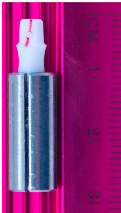
Fig. 1. Ceramic dental implant mounted in the cylindrical steel jacket. The red marker line indicates the side to be bent during loading. (For interpretation of the references to colour in this figure legend, the reader is referred to the web version of this article.)
