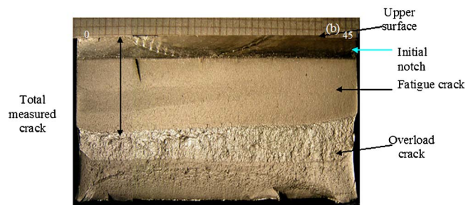
FIG. 3. (a) Crack-front profile, as determined from surface, bottom, and actual measurements. Surface data are processed assuming a thin skin and the proposed approximation. Note the excellent agreement between the actual crack-front profile and its estimates using bottom measurements and the proposed approximation for surface measurements. (b) Specimen (4) [of (a)] after being open in the laboratory.
