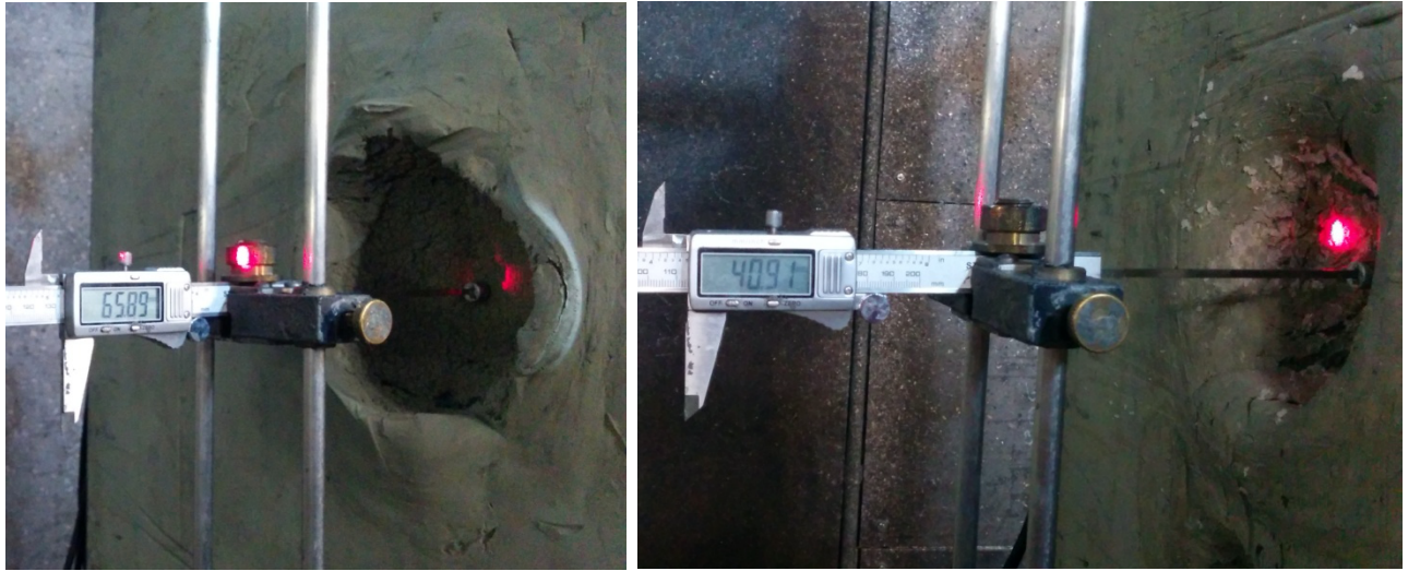
Figure 1. A comparison between the crater depths, caused by the shockwaves of a stopped FN MAG bullet, between an armor layer without a anti-trauma element (left) and an inverse-freezing anti trauma element (right). The measured depths are 66 mm and 41 mm respectively.
